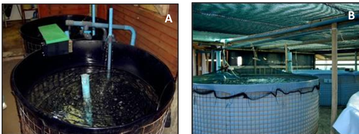
Figure 7: A) Larval rearing; and B) Nursery tanks in a land-based facility.
