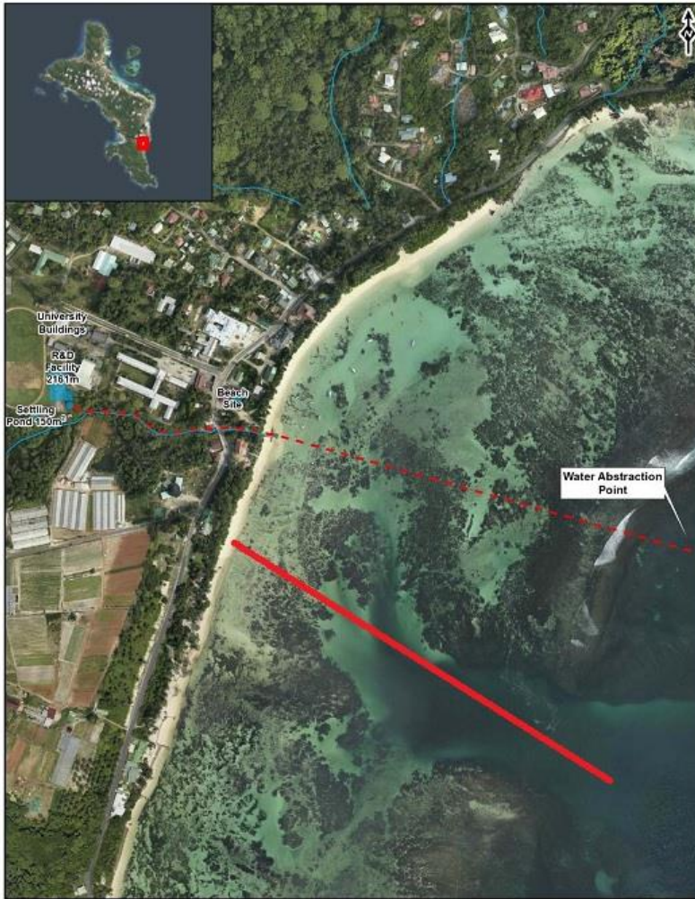
Figure 24. The proposed re-routing of the pipeline indicated by the solid red line
