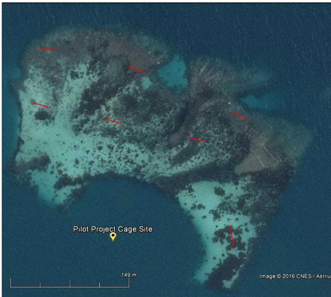
Figure 26. An example of a survey design for monitoring coral reef habitat (or seagrass). Transects are indicated by red lines.
