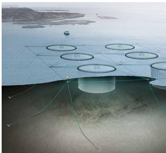
Figure 2. Circular high-density polyethylene cages likely to be used within Aquaculture Development Zones (ADZs).
