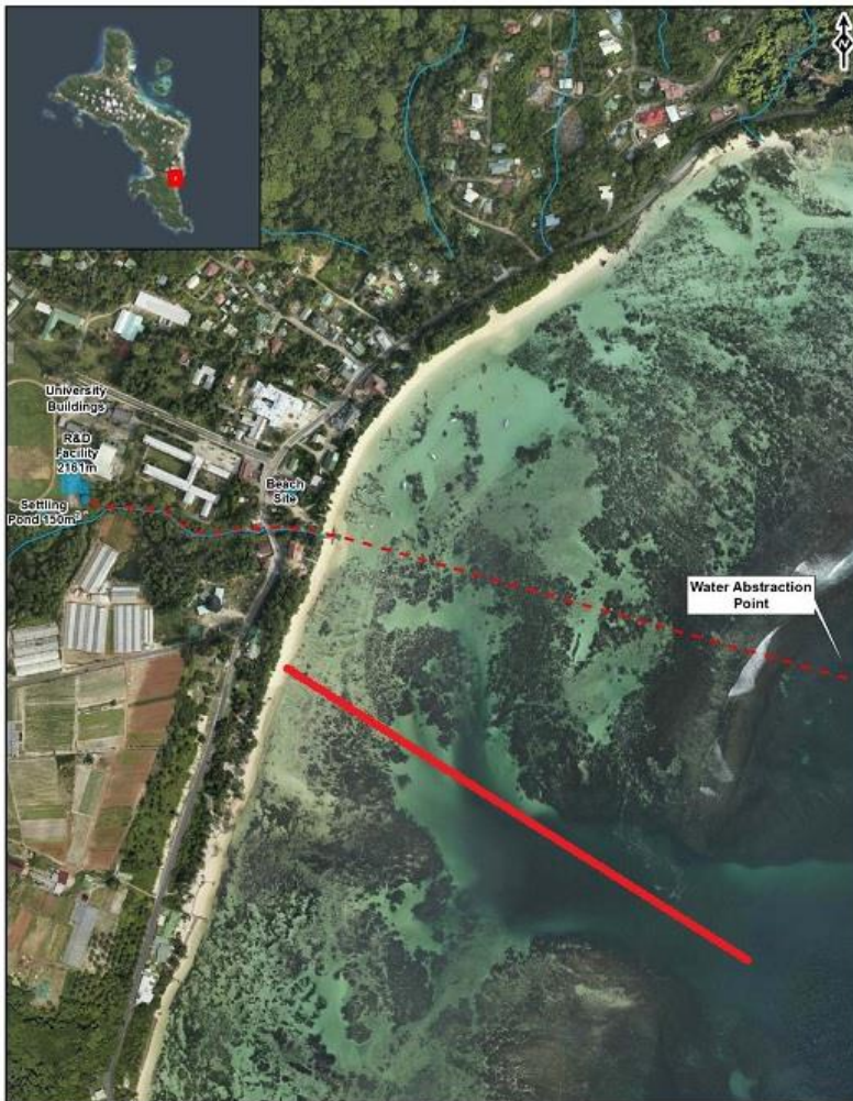
Figure 66: The proposed re-routing of the pipeline indicated by the solid red line
