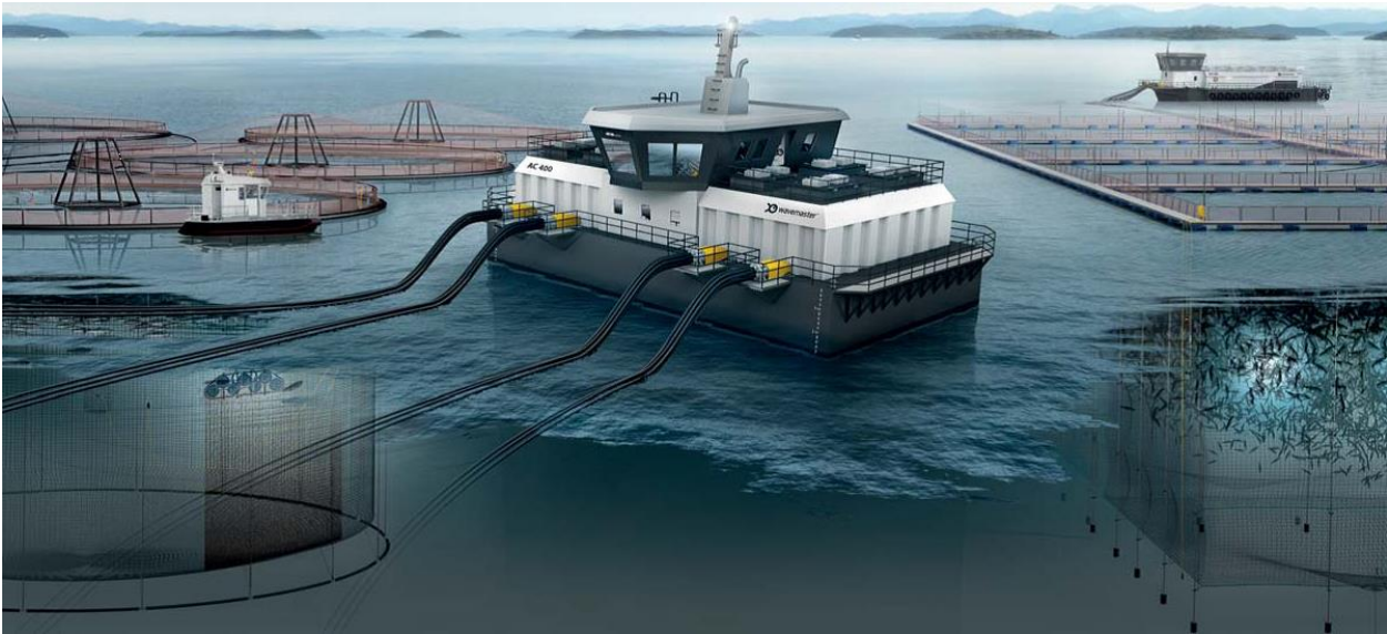
Figure 17: Example of an AKVA Feed Barge
