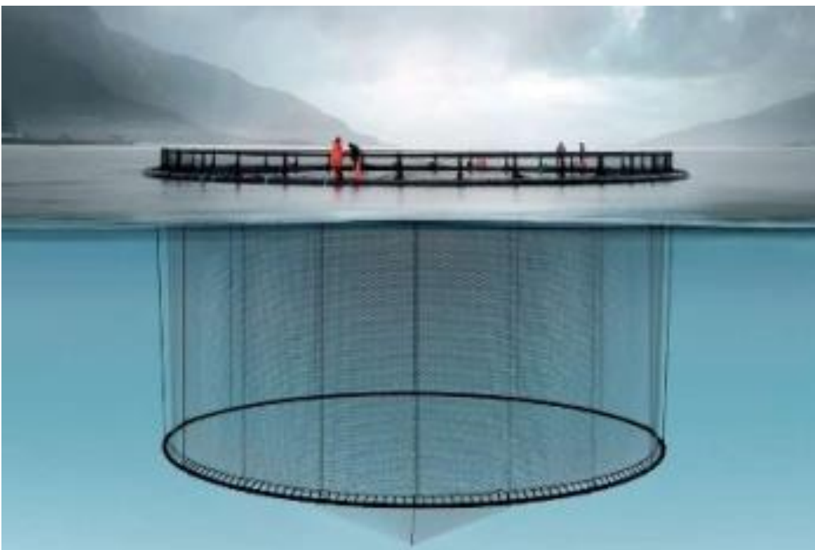
Figure 6: Typical Cage Structure
