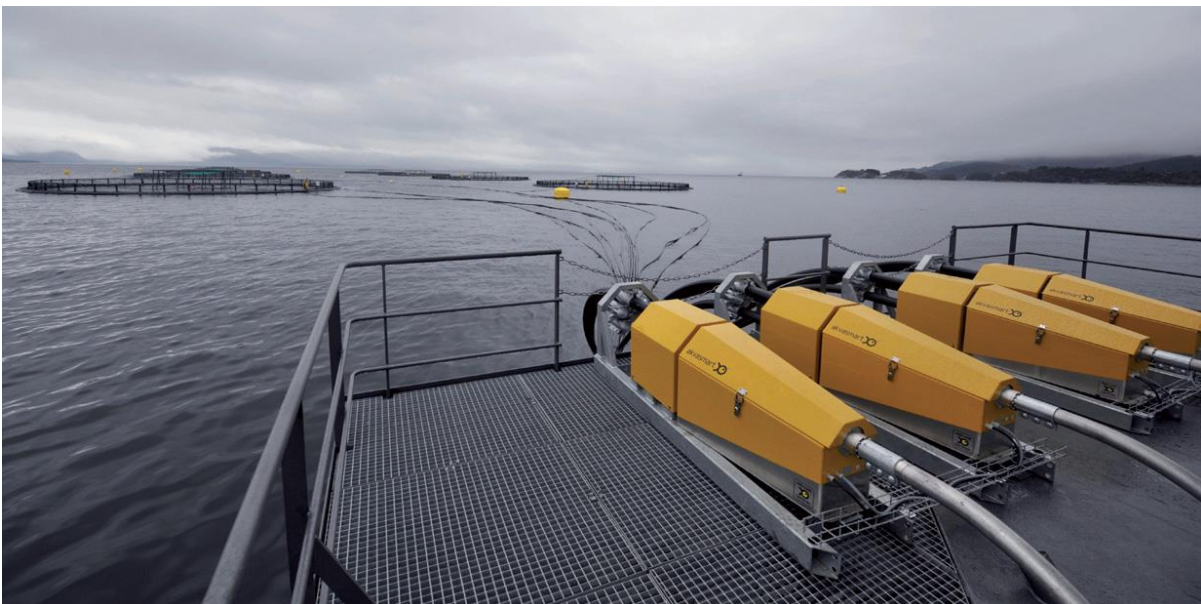
Figure 7: Example of an automated AKVA Feeding System
